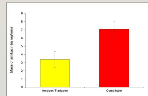
In addition, the output rate of amikacin was higher with the Combihaler chamber compared to the Aerogen T-adaptor (7.1±0.2 mg/min vs 3.4±0.2 mg/min).
